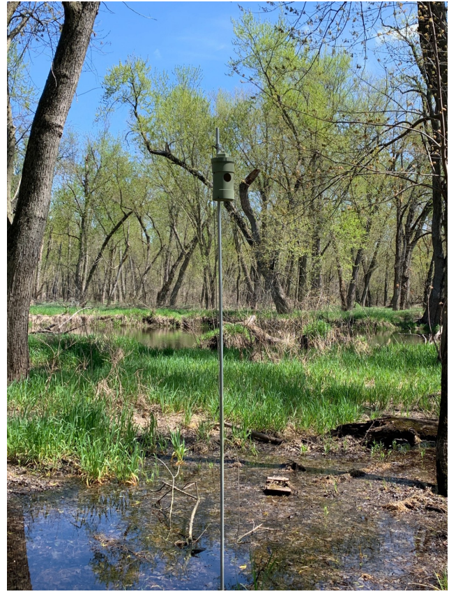
Fig. 2. A flood resistant PVC nest box designed to be elevated above potential flood waters at our study site in Scott County, Iowa. It is mounted on a 3 m electrical conduit pole.
