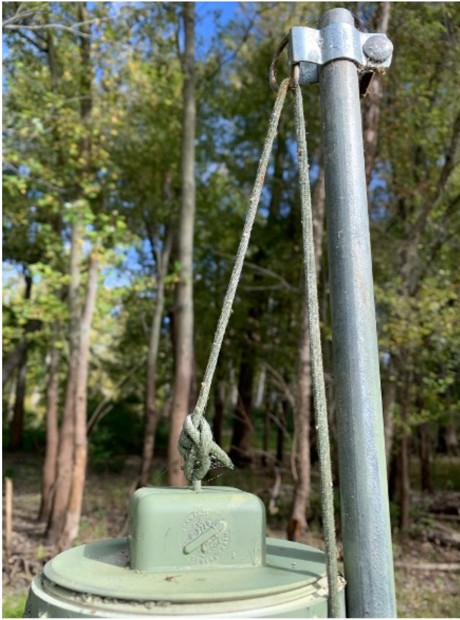
Fig. 5. A conduit hanger is attached at the top of the electrical conduit pole and has a ring through which the paracord is pulled up and down to check the nest box contents and then to return it to its resting location at the top of the electrical conduit pole.
