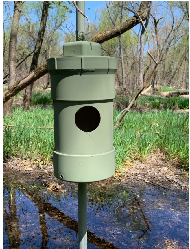
Fig. 4. A flood resistant PVC nest box attached to the electrical conduit pole showing the paracord attached to the screw-eye hook on top of the nest box. The nest box is raised above potential flood waters and then lowered to check the nest contents using the paracord.
