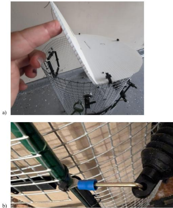
Fig. 2. Photos of details of the remotely closing trap. (a) A corrugated twinwall plastic sheet was attached to the top of the trap with zip ties. The bottom wall of the plastic sheet was sliced to create a flap that allowed a bird feeder to be lowered in and raised out of the trap. A small rectangle was cut out to allow the feeder hanger to be passed through the plastic sheet to suspend the feeder/trap combination from a shepherd's hook. (b) Close-up of connecting rod and forked wire connector holding the door in the open position.
