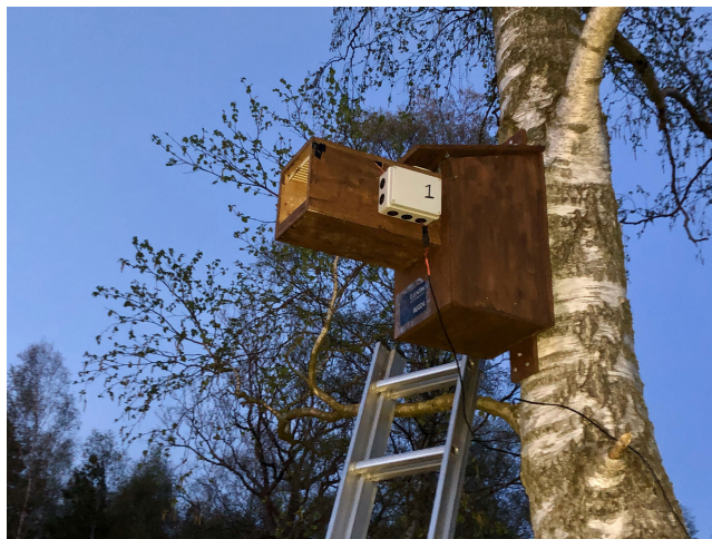
Fig. 2. A “smart” trap fitted to a nestbox, with a PVC box housing the electronics and a power cable leading to a car battery situated at the base of the tree.
