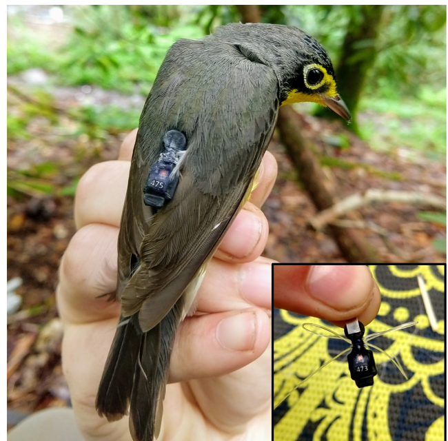
Fig. 1. Light-level geocator (FL6057 fLight Lotek Wireless) attached via leg-loop harness to an adult male Canada Warbler ( Cardellina canadensis ) in the Monongahela National Forest, West Virginia, USA, in 2020. Inset shows the geocator pre-deployment with the harness made from 0.5 mm elastic cord. Photo credit: Stephanie Augustine.
