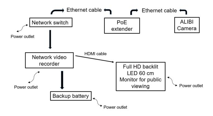
**APPENDIX 2.** Diagram of the components of the camera and equipment installation.
